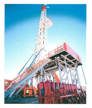
**DRAWWORKS:** GES 1,600 HP AC Drawworks, grooved for 1-3/8" drill line, driven by 1500 HP continuous, 1830 HP intermittent AC drive motor.
