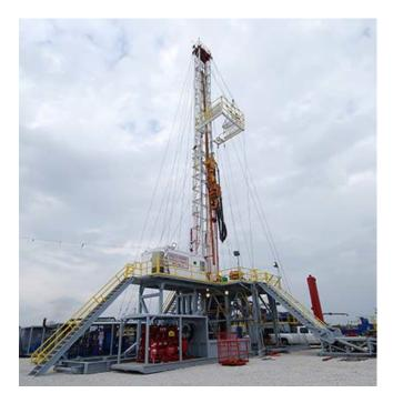
**DRAWWORKS**: CROWN ENERGY TECHNOLOGY MODEL CE 750 SD 750 HP, GROOVED FOR 1 1/8" DRILLINE, POWERED BY 2 DETROIT SERIES 60 MOUNTED ON A 4 AXLE TRAILER.
