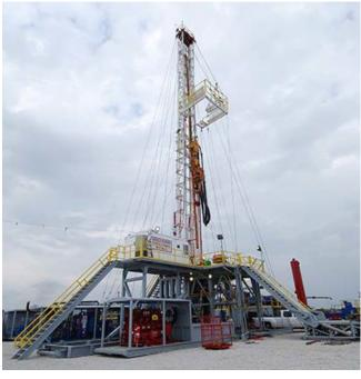
**DRAWWORKS:** CROWN ENERGY TECHNOLOGY MODEL CE 750 SD 750 HP, GROOVED FOR 1 1/8" DRILLINE, POWERED BY 2 DETROIT SERIES 60 MOUNTED ON A 4 AXLE TRAILER.
