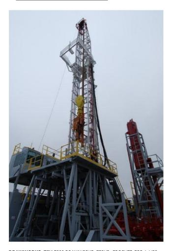
**DRAWWORKS:** TSM 7000 DRAWWORKS, 750HP, GROOVED FOR 1 1/8" DRILL LINE, POWERED BY 540HP CAT C-16, W/ALLISON CLT-6061 AUTOMATIC TRANSMISSION, RIGHT ANGLE DRIVE, DEAD LINE ANCHOR, ALL MOUNTED ON AN OILFIELD SKID
